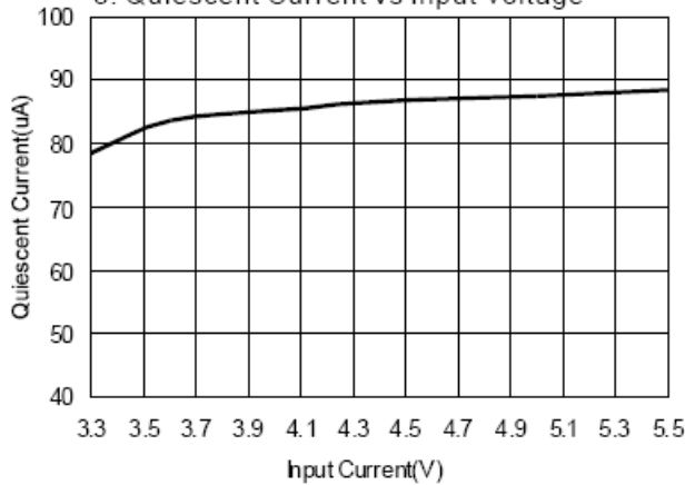
3. Quiescent Current vs Input Voltage
